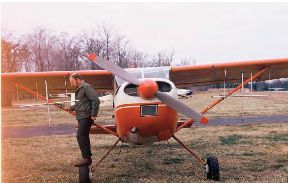
Matt Perry checking tracking antennas after refueling at Lee Airport, Annapolis, in 1973
