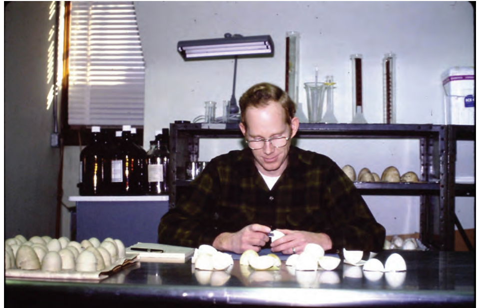
Patuxent scientist, Stan Wiemeyer, measuring the thickness of bald eagle eggshells with a micrometer, early 1970s.
