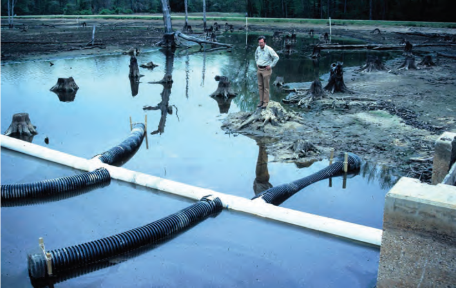
Holly Obrecht inspecting a new beaver baffle design by University of Maryland students in drained Knowles 1 impoundment, 1992.
